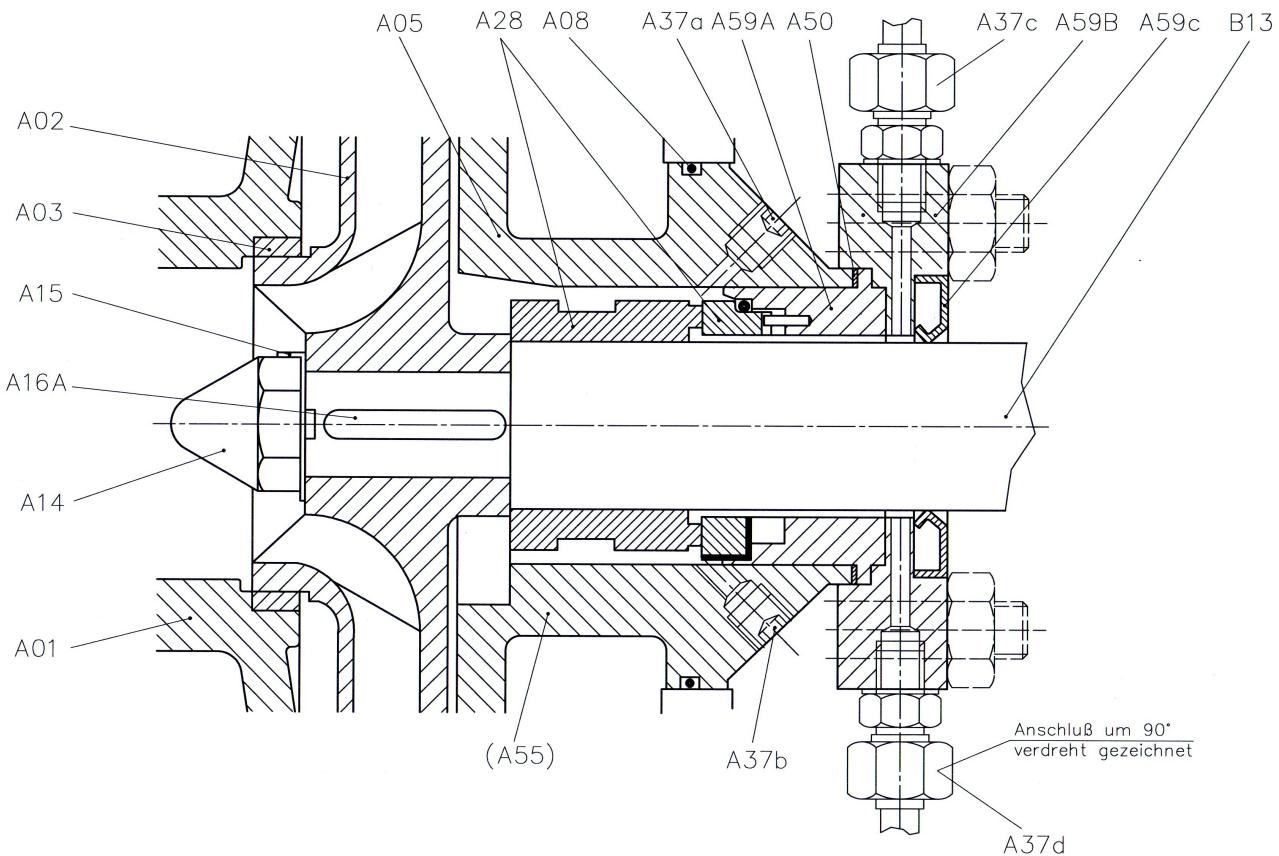
**ATTENTION:** The plug screw pos. A37d must be unclosed during the filling of the sealing medium box. Until the sealing medium discharge at the plug screw you must let open the outlet. So you prevent the creation of air cushion. Then close the plug screw again.
