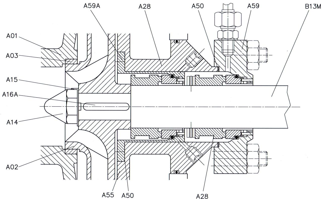
The sealing room will be flushed non-pressurized with the sealing medium.
