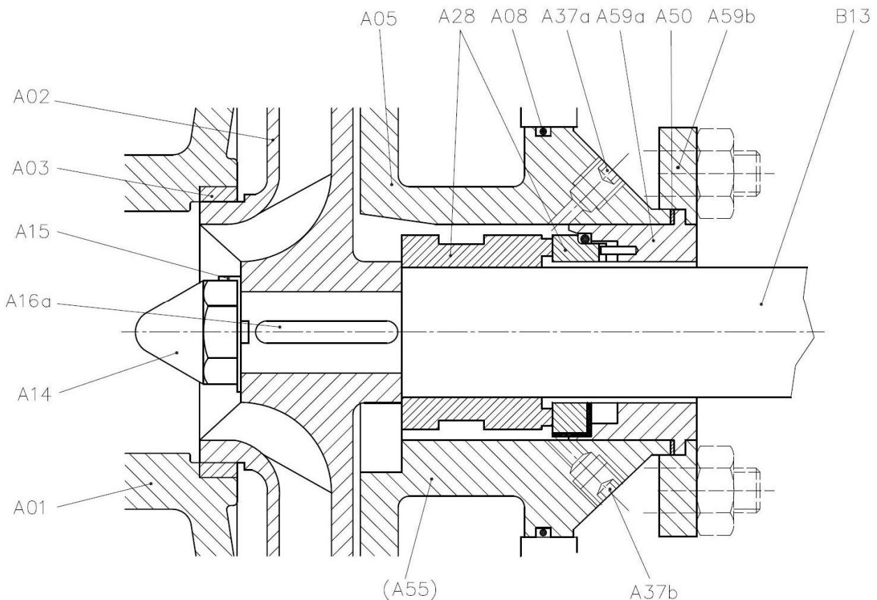
The sliding faces are pressed against each other by means of spring force, thus preventing the opening of the seal at stand-still. The seal faces are statically sealed against the housing and the shaft by secondary seals. With the entry of the pumped medium into the minimal sealing gap a lubricating film is generated and the sealing effect is thus obtained.
