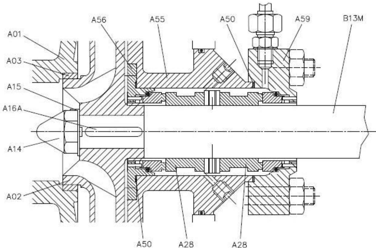
The pressure in the cavity between the two seals have to be ca. 1 bar over the working point of the pump. So it can be guarantee that the sealing faces are flushed only with pure medium.
