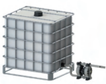
Pump installed below head (positive suction)
