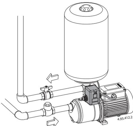
With EASYMAT it is easy to create a variable speed system starting from an existing fixed speed system without disturbing the existing pipe-work.
